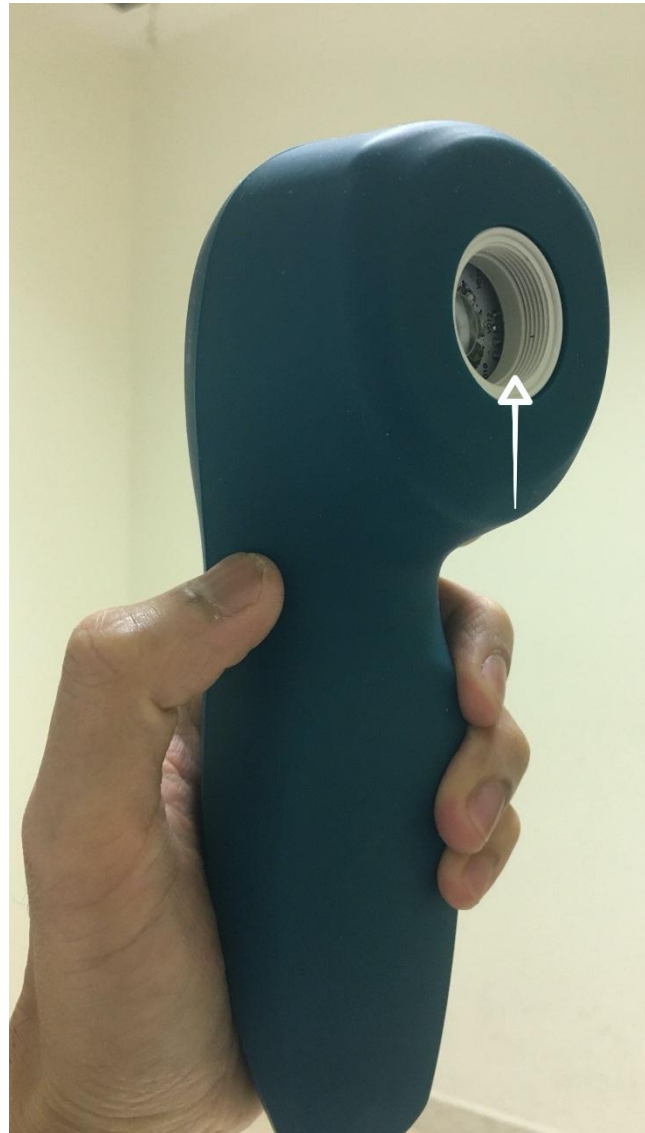
Figure 4 The cluster probe consisted of an aperture of 4 cm 2 and a concave tip (arrow).
